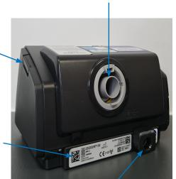
Filter and circuit attaches here
